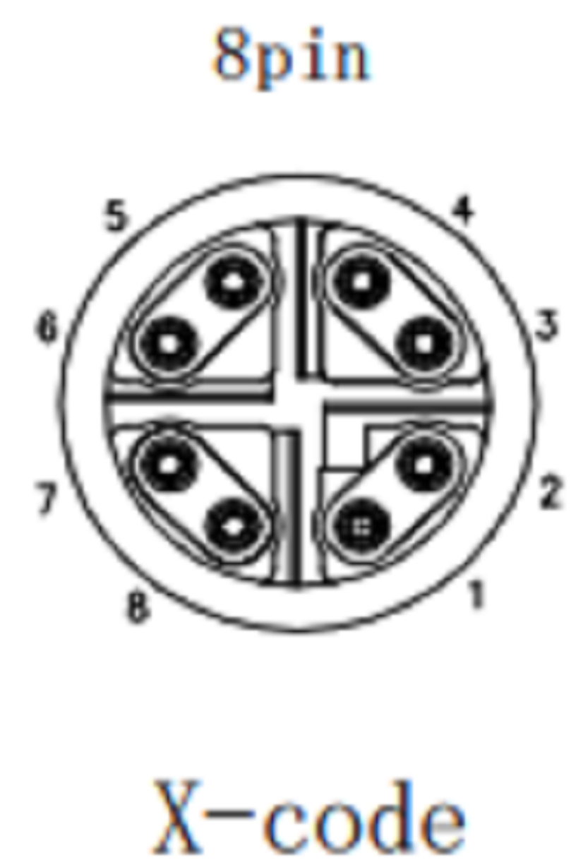
Pin assignment front view/针位分布前视图
